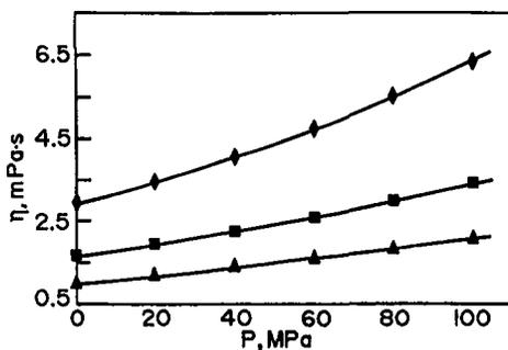
Fig. 6. Dynamic viscosity  $\eta$  versus pressure  $P$  at various temperatures  $T$ , for composition  $x_w=0.3$ ,  $x_d=0.4$ ,  $x_p=0.3$  (◆: 303.15 K, ■: 323.15 K, ▲: 343.15 K).
