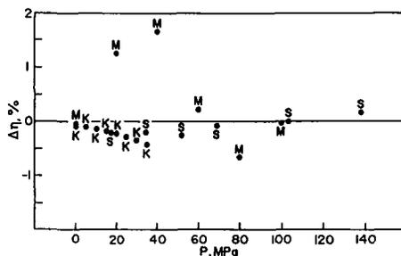
Fig. 2. Deviation  $\Delta\eta$  of the literature data for the viscosity of water from the equation:  $\eta = a + bP + cP^2$  ( $T = 303.15$  K). K, Ref. 7; S, Ref. 8; M, the present work, Ref. 2.
