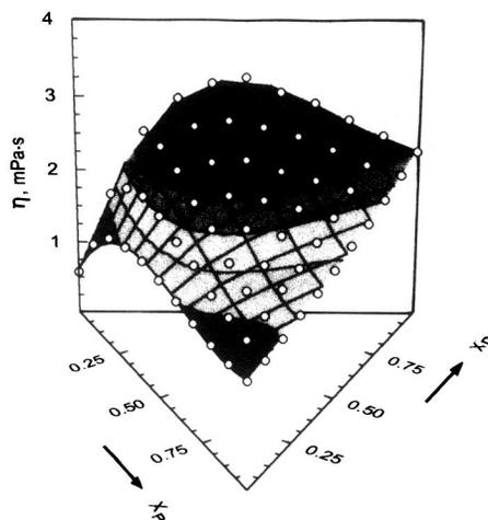
Fig. 10. Surface  $\eta(x_w, x_d, x_p)$  in the ternary diagram at  $P=40$  MPa and  $T=323.15$  K.
