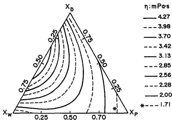
Fig. 11. Isodynamic viscosity lines in the ternary diagram at  $P=0.1$  MPa and  $T=303.15$  K.
