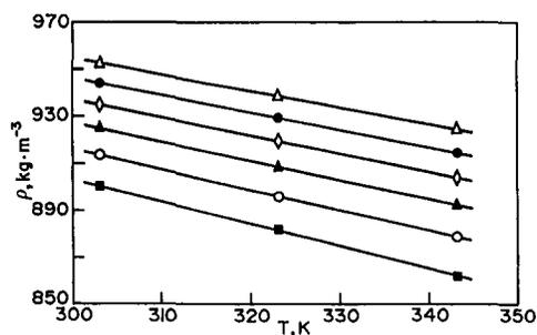
Fig. 5. Density  $\rho$  versus temperature  $T$  at various pressures  $P$ , for composition  $x_w=0.3$ ,  $x_d=0.4$ ,  $x_p=0.3$  ( $\blacksquare$ : 0.1 MPa,  $\circ$ : 20 MPa,  $\blacktriangle$ : 40 MPa,  $\blacklozenge$ : 60 MPa,  $\bullet$ : 80 MPa,  $\triangle$ : 100 MPa).
