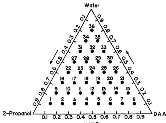
Fig. 3. Points representative of the three pure substances, the three binaries, and the ternary in the ternary diagram (versus mole fraction).
