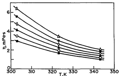
Fig. 7. Dynamic viscosity  $\eta$  versus temperature  $T$  at various pressures  $P$ , for composition  $x_w=0.3$ ,  $x_d=0.4$ ,  $x_p=0.3$  (■: 0.1 MPa, ○: 20 MPa, ▲: 40 MPa, ◇: 60 MPa, ●: 80 MPa, △: 100 MPa).
