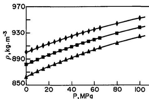
Fig. 4. Density  $\rho$  versus pressure  $P$  at various temperatures  $T$ , for composition  $x_w=0.3$ ,  $x_d=0.4$ ,  $x_p=0.3$  ( $\blacklozenge$ : 303.15 K,  $\blacksquare$ : 323.15 K,  $\blacktriangle$ : 343.15 K).
