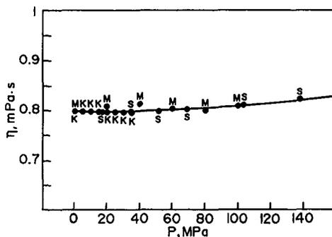
Fig. 1. Dynamic viscosity  $\eta$  of water versus pressure at  $T = 303.15$  K ( $-\eta = a + bP + cP^2$ ). K, Ref. 7; S, Ref. 8; M, the present work, Ref. 2.
